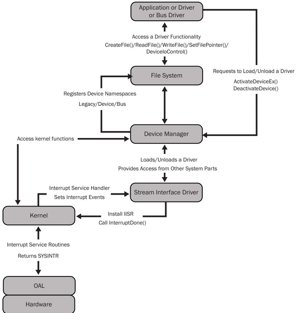
FIGURE 6-4 Stream driver architecture
