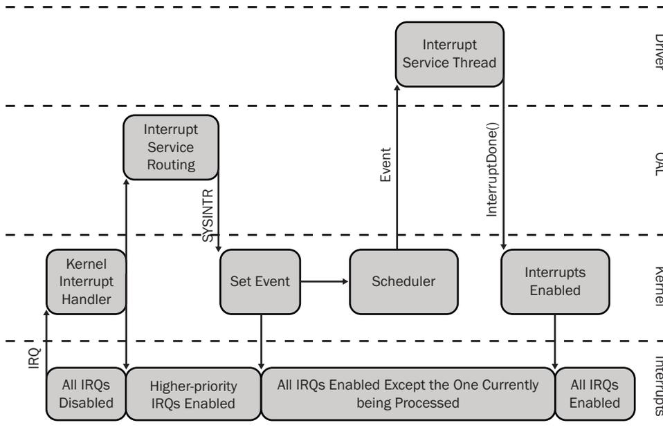
**FIGURE 3–9** Interrupt handling
