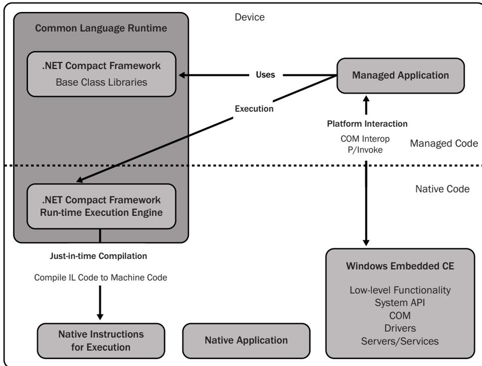
**FIGURE 9-1** Native and managed application code architectures on a device
