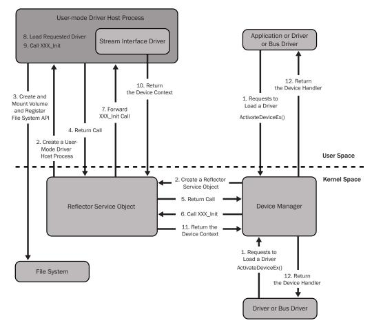
FIGURE 6-5 A user-mode driver loading process
