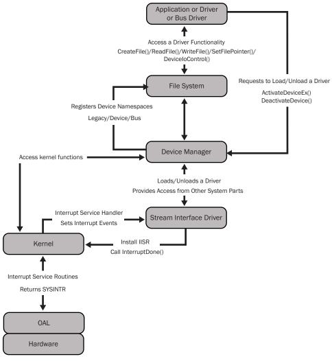
FIGURE 6-4 Stream driver architecture
