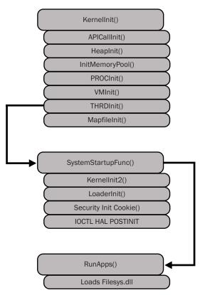
FIGURE 7-2 System startup process KernelInit()->RunApps()
