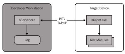
FIGURE 10–13 Windows Embedded CE Stress Tool architecture
