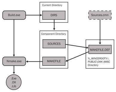
FIGURE 4–3 Components and modules build process
