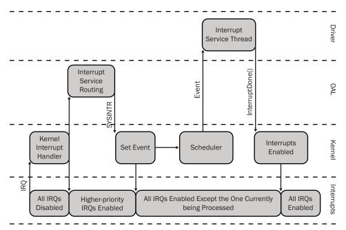
FIGURE 3–9 Interrupt handling
