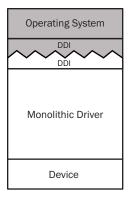
FIGURE 6–3 Monolithic driver architecture
