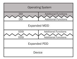
FIGURE 6–2 Hybrid driver architecture
