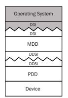
FIGURE 6–1 Layered driver architecture
